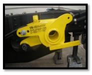
21. Carefully and gradually lower the axle with the jack until the hole in the left hanger lines up with the hole in the Sulastic spring. Then, insert and tighten the bolt. Repeat this step for the right Sulastic spring.
