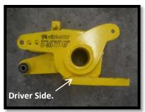
13. The Sulastic springs are labeled as to either the driver or passenger side of the vehicle. If not please see the figure.
