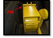
b. Now raise the hydraulic jack in order to open the sulastic and hits the stop member During this step check that nothing interferes with the operation of the sulastic in given case please give us a call to advice you and if possible provide photos as reference.
