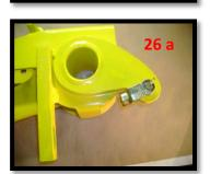
b. Afterwards, screw the rod into the yoke end about one inch. In order to tighten the rod into the yoke end, place two nuts at the other end of the rod and tight one nut while you hold the other one in place. Once the rod is tight to the yoke end remove the two nuts and tight the nut you place in the step a. to secure the rod in place.
