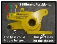
14. Select the hole on which you will mount the sulastic to the leaf springs . This is a very important step because it will determine the inclination of the sulastic which will avoid any interference with the sulastic.
