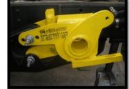
22. Now, using a torque wrench, carefully tighten each nut to the required torque value, as indicated in the manufacturer's manual.
