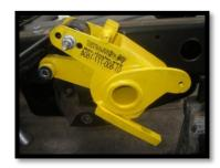
20. At this time, each Sulastic spring should be attached only to the leaf spring with nut and bolt. You are now ready to attach each Sulastic spring to its hanger.
